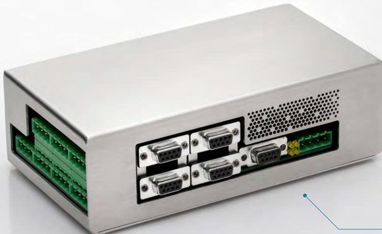
Thanks to the cyber® motor select switch, up to four motors from WITTENSTEIN cyber motor's industrial small servo drive system can be selectively controlled using a single servo drive.
